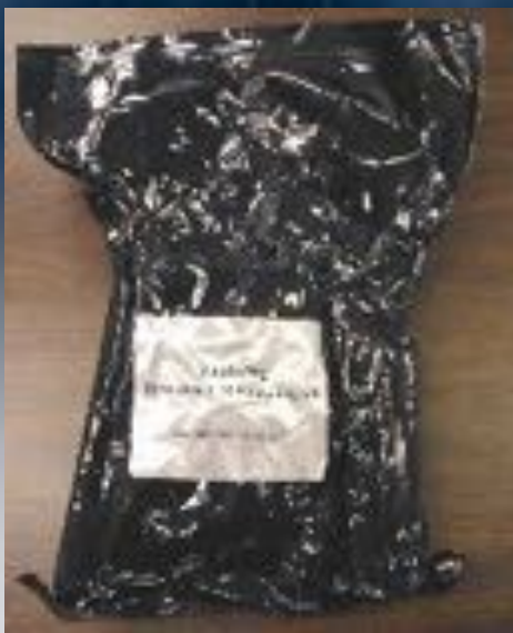
Mylar Vacuum Sealed CB Sampling Kit Weight: 2.6 lbs Dimensions: 13 x 7 x 3"
