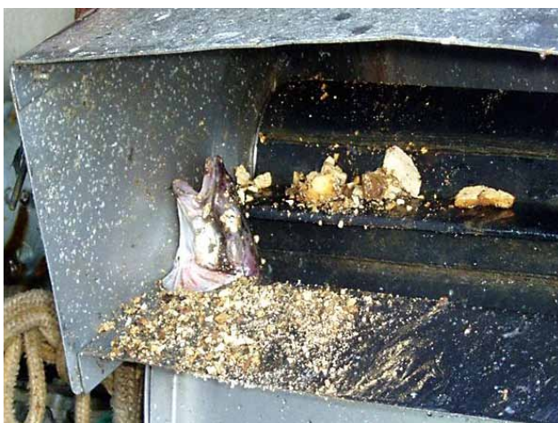
Figure 37: Small lumps of sulfur mustard in the fish conveyor belt on board a fishing vessel. Since it could not be ruled out that some of the particles actually might be explosives, they had to be emergency-relocated ( cf. Chapters 3.2.3.3 & 4.3.1) (Picture source: Maritime Surveillance Centre South on Bornholm).
