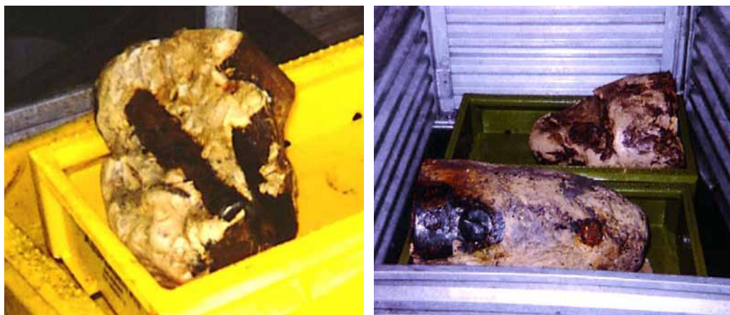
Figure 39: Lumps of solidified sulfur mustard trawled up with a catch. Since they contain explosives (left - bursting charge tube with about 15 kg of explosives visible), they were emergency-relocated ( cf. Chapter 3.2.3.3) (Picture source: Maritime Surveillance Centre South on Bornholm).
