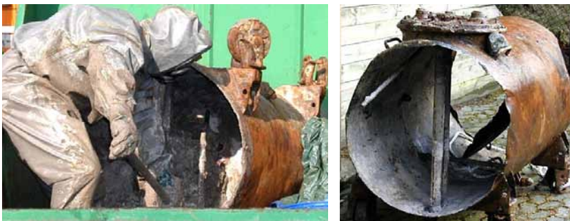
Figure 43: A 900 L container of unknown origin ( cf. Figure 28) with 1,057 kg of Clark I-type chemical warfare agent mixture was found in a warehouse in the port of Nexø in 2001 ( cf. Annex 7.2 - Table 7). It was decontaminated and the contents disposed of in a disposal facility (Picture source: Maritime Surveillance Centre South on Bornholm).
