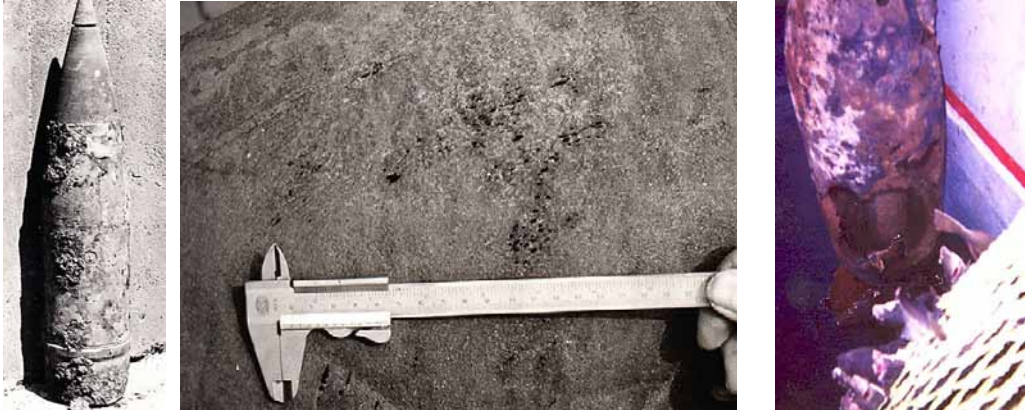
Figure 30: Corroded chemical munitions recovered from the Baltic Sea in recent decades. Left to right: 15 cm Tabun shell, 1960; KC250 Tabun bomb, 1960 (Picture source: Internal Documentation State Office for Civil Protection – bomb disposal services); empty KC250 bomb (Picture source: Maritime Surveillance Centre South on Bornholm).
